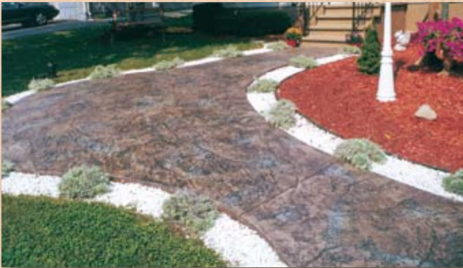
Penn Blue highlighting color was used on a Sandstone Integral color base, along with Charcoal Release to achieve an appearance with the Jumbo Stone Texturing pattern that individualizes this project.
